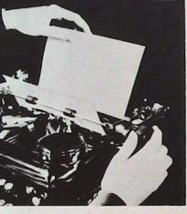
THE NEW PAPER LOCK A flip of the finger, and the lock opens, permitting the paper to be inserted straight without adjustment. As paper lock closes, it rolls sheet firmly against the cylinder. Withdrawal of the paper automatically opens this new paper lock.
