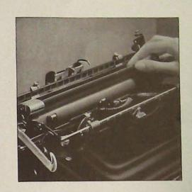
A new pressure-adjuster, conveniently placed just above the keyboard, regulates the machine for multiple copy work and also for fill-in work when the degree of inking must be matched. When one to six copies are to be made, this lever need not be moved at all . . . with the adjuster, as many as fifteen clean cut copies can be made! Yet, greater number of copies means no increase in writing effort because of the dial control . . . a feature that also saves ribbon wear.
