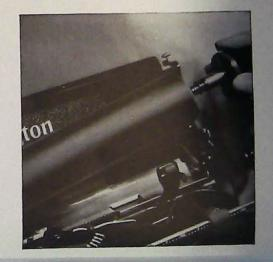
The regular platen on the NEW REMINGTON NOISELESS can be instantly removed and a card platen-with a special clip to hold the card-inserted in its place. As you can see, the platen on this model is so designed that the cards can be fed as in regular letter writing or by front feeding, permitting writing on both top and bottom edges of cards. Card platens are available at small extra cost in many widths and may be designed to meet your specific requirements.
