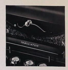
This new tabulator rack carries an inbuilt stop for every space. Stops cannot work loose, fall out or drop down into the machine. The operator doesn't have to hunt around for the correct tabulator stop . . . it's always in position right at the desired point in the machine. As explained above, control of stops is simplicity itself—clearing and setting being accomplished through control keys.
