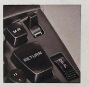
RIBBON COLOR SELECTOR The Ribbon Color Selector is on the upper right of the keyboard. Move it up to the black or down to the red position for typing in the desired color. When typing stencils, set the Selector at the middle position where the keys will not leave an inked impression.
