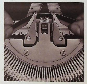
MANUAL RIBBON REVERSE The ribbon on your Smith-Corona reverses itself automatically when it nears the end of the spool. To reverse the ribbon manually, just flick the Ribbon Reverse (RIB REV) Lever at the left of the keyboard.
