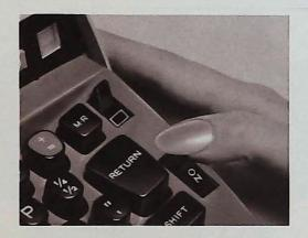
ON-OFF SWITCH Plug the typewriter cord in, turn the switch to ON, and you're ready to go. The switch is located just to the right of the typing keys. A handy indicator on the upper right front panel lights whenever your machine is on. Make sure you always turn the typewriter off when it is not in use.
