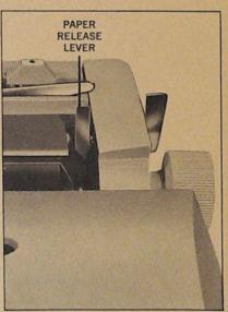
To insert properly, place the paper against the paper table behind the cylinder with your left hand. The paper should rest lightly in this slot with left edge flush against the paper guide as your right hand slowly turns the right cylinder knob to feed the paper around the cylinder.
