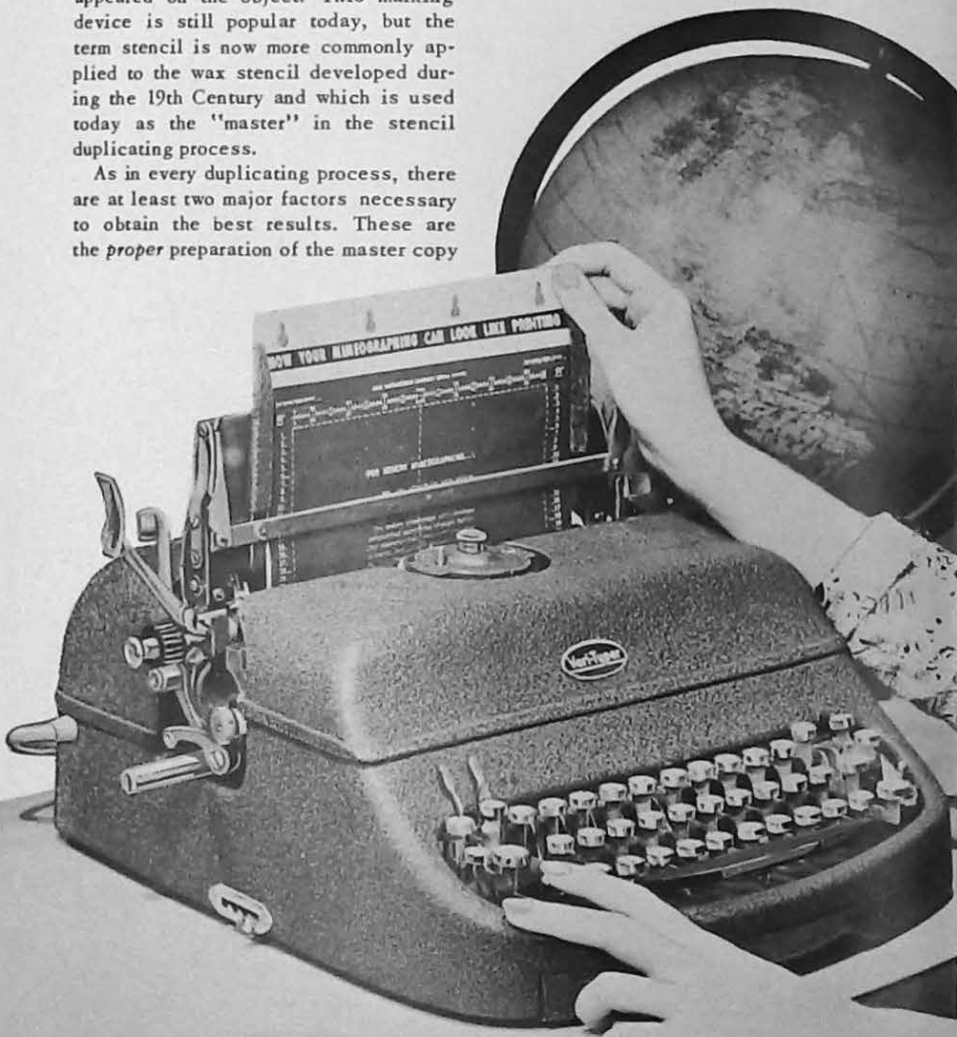
The typing action of the Vari-Typer is illustrated above. The impression of the hammer against the type can be regulated to produce copy that is uniformly sharp and clear.
