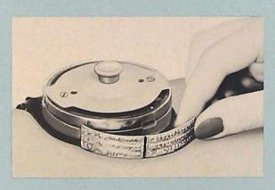
It takes less than a second to change Type Fonts in the VariTyper machine. Two Fonts are in use at one time so that matching italics, bold faces, or special symbols can be inserted in the copy as the "typing" operation progresses. Additional Type Fonts are inserted in the machine in a second or two. The instantly changeable-type feature of the VariTyper machine is coupled with instantly variable spacing to match the individual size and style needs of the Font selected.
